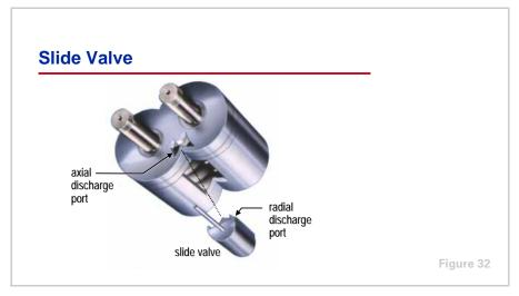
The position of the slide valve along the rotors controls the volume of refrigerant vapor being delivered by the compressor, by varying the amount of rotor length actually being used for compression.
